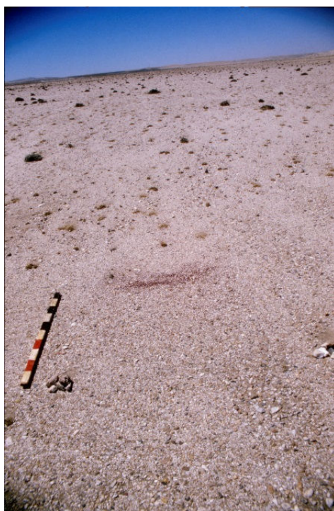
Figure 21. Dispersal of the garnet bedload creep tracers by aeolian processes. By 05/01/88 the initial line of garnet grains had been transported about 1 to 1.5 m to the north across the stone pavement. The original starting point is marked by a pile of stones near the scale. Southerly wind flow from bottom to top, scale 1 m
